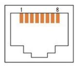
Pin 5: RS485 A line Pin 4: RS485 B line Pin 8: RS485 GND and shield
